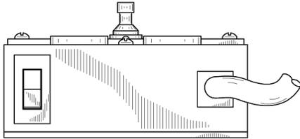
The rear panel houses the main power rocker switch and the power cord. A light in the switch will glow red any time the switch is in the On position and the power cord is plugged into a properly functioning power outlet.
