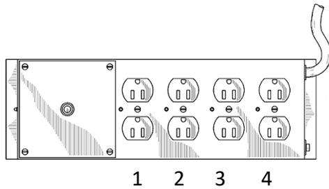
The top panel of your RS-4 provides four duplex receptacles, each with a dedicated red LED. This instruction manual references each receptacle, and its dedicated LED, by number 1 thru 4. Receptacle number 1, first to turn on, and is next to the push button switch. Receptacle number 4, last to turn on, and is next to powercord.
